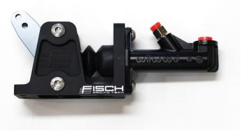
Install the two screws that hold the master to the base This may be easier with the brake line fitting removed
