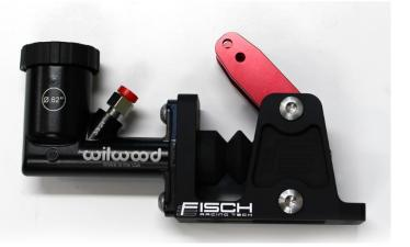
Install the two screws that hold the master to the base This may be easier with the brake line fitting removed
