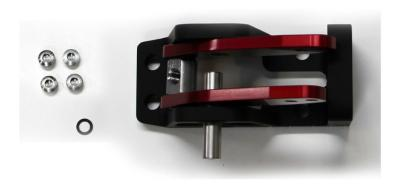
Install the smooth pivot pin into the lower hole on the base The last 2 nylon washers go between the arms and the base
