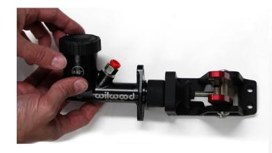
Turn the master into the threaded pivot pin until there is about 10mm sticking past You can also do this by turning the piston, rather than the full master
