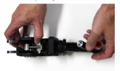
Turn the master into the threaded pivot pin until there is about 10mm sticking past You can also do this by turning the piston, rather than the full master
