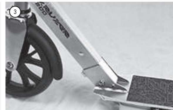
IF LOCKED CORRECTLY, THE FOLDING MECHANISM WILL NOW FEEL SECURE WITH LITTLE TO NO PLAY. IF IT SEEMS LOOSE, PULL THE BARS UP RAPIDLY UNTIL YOU HEAR A CLICK - REFER TO TROUBLESHOOTING STEPS.
