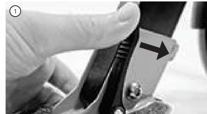
TO FOLD AND UNFOLD YOUR KRUIZER SCOOTER, PRESS IN THE LOCKING LEVER FIRMLY.
