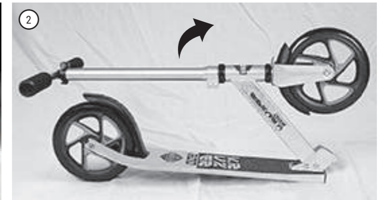
THE FOLDING MECHANISM WILL RELEASE ALLOWING THE SCOOTER HANDLEBAR TO EXTEND INTO THE UPRIGHT POSITION
