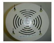
2. Remove the 4 screws from the base plate
