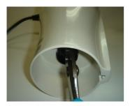
3. Grasp the motor clutch firmly with pliers
