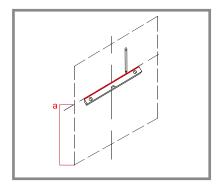
**Step 02:** Mark the punching position on the wall with a pencil. use level gauge make sure the hole at the same level.
