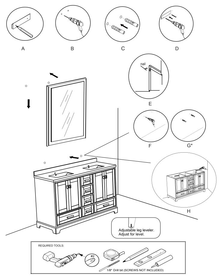
\*SECURE SCREW TO STUDS WHEN POSSIBLE
