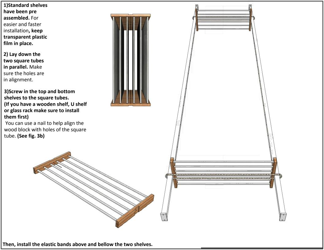
1)Standard shelves have been pre assembled. For easier and faster installation, keep transparent plastic film in place.
