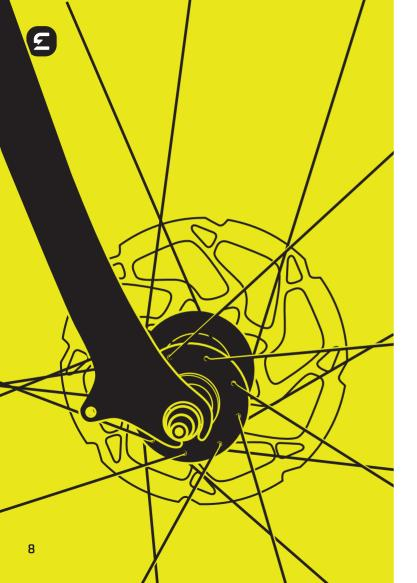
Remove the black plastic protector from the fork and the orange plastic protector from the brake pads, making sure not to press the front brake lever.
