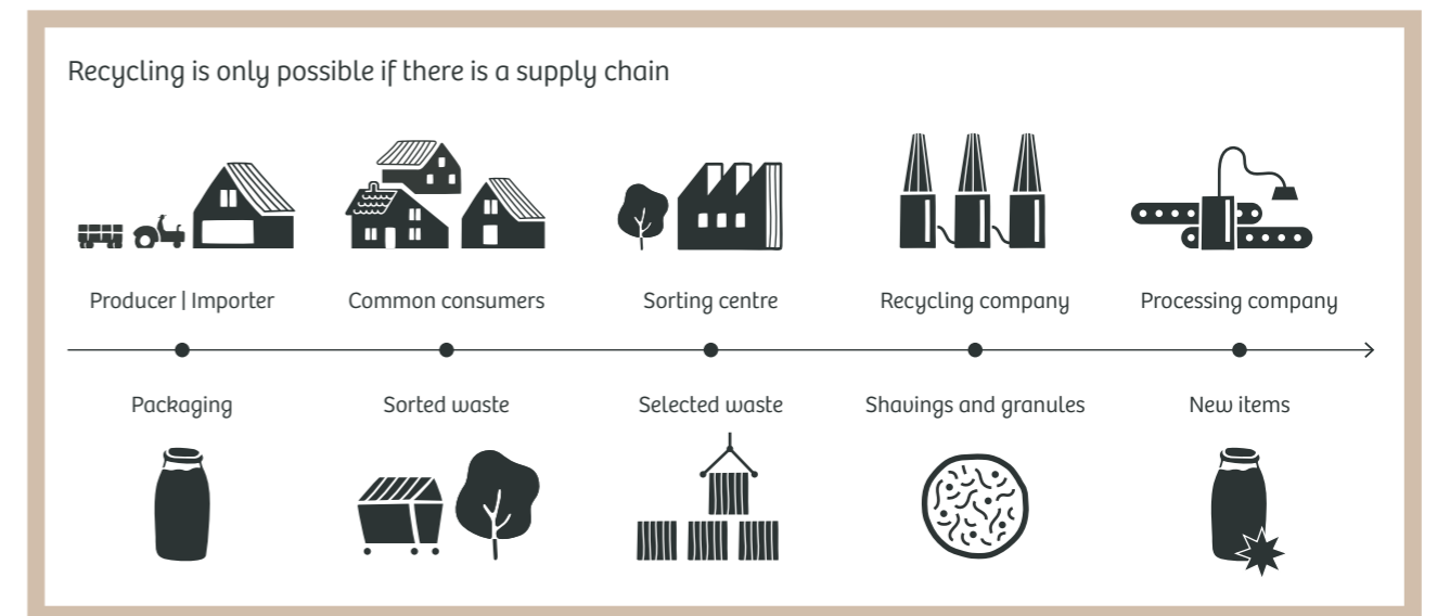
Plastic recycling supply chain diagram (CONAI guidelines)
