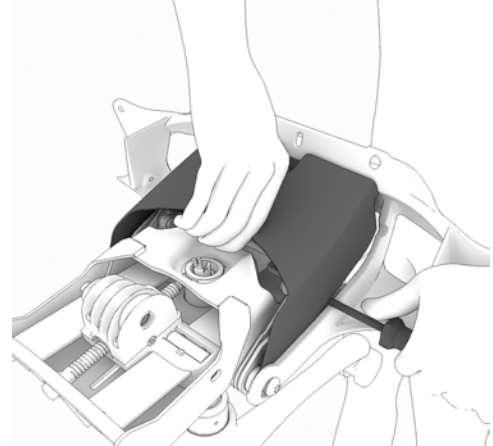
40. Slide flat blade screwdriver along side of rear tilt cover and pry off.
