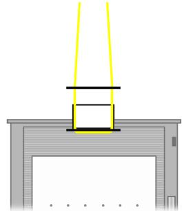
of the spigot. Make sure that the adjustable flue damper is not fouled by the lifting rope. Feed a suitable lifting pole though the strap, looping the rope around the pole until the correct length is achieved. The rope is at the correct length when, with the pole on their shoulders and the rope taut, the knees of the people lifting it are slightly bent. The stove
