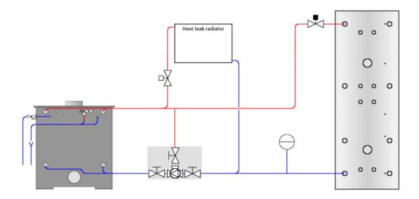
Unvented circuit on thermal store – PRV can be installed on pipe work behind stove, there must be no restrictions between PRV and stove.
