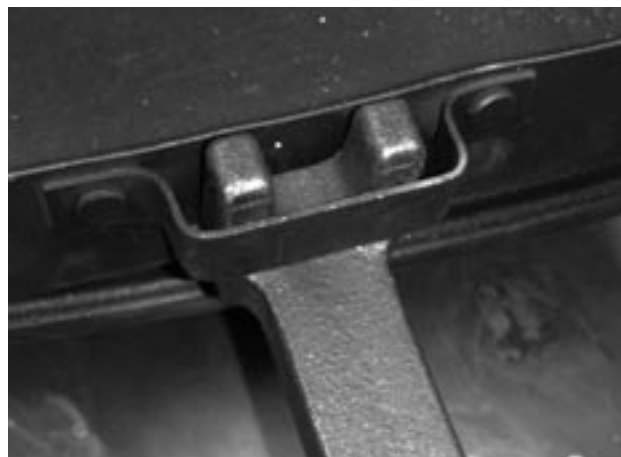
The forked end of the tool is inserted underneath the ash pan grip as shown above to create the ash pan handle.
