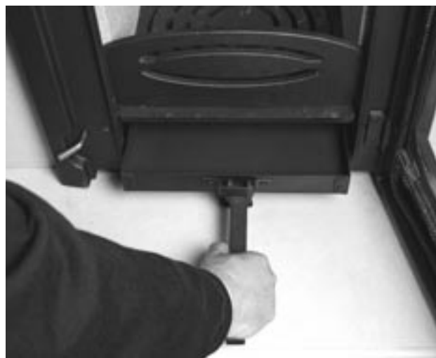
The forked end of the tool is inserted underneath the ash pan grip as shown above to create the ash pan handle.
