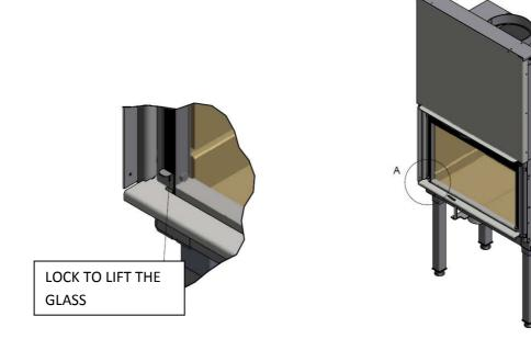
A lock to lift the glass is located on each side of the door in order to facilitate the retractation. During this operation, do not pull the door but help the opening & closing operations by pressing on the lift lock.
