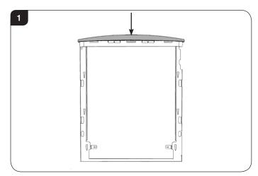
3.3 Fasten the Cast Top using the 2 fixing screws provided, see Diagram 2.
