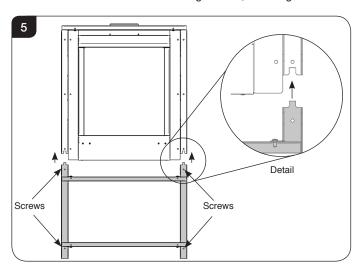
2b.5 Mark the position for the 4 fixing screws, see Diagram 5.
