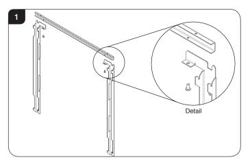
2a.3 Offer the wall mounting brackets to the appliance and position so all the interior edges sit flush with the edges of the appliance flange, see Diagram 2.
