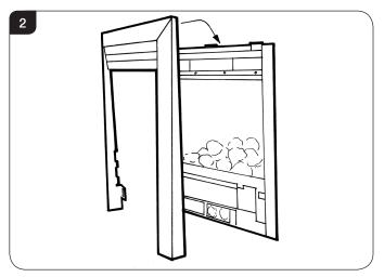
2.2 Secure frame at base with fixing screws as shown to ensure rigid fixing, see Diagram 3.
