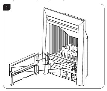
3.2 Place ash pan cover into position at base of the front, see Diagram 5.
