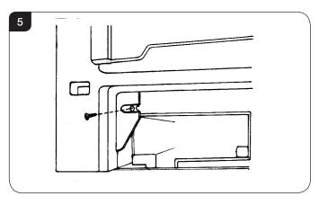
2.8 Replace the door by slotting the hinge pins into the hinge blocks.
