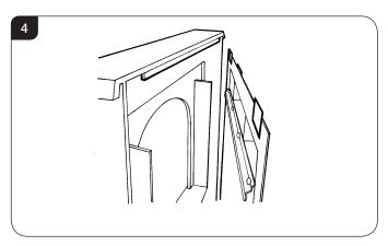
2.7 Secure to both sides of the appliance with the 2 pozidriv screws supplied, see Diagram 5.
