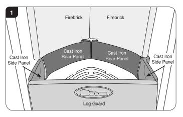
The Firebricks and cast iron rear panels do not need to be removed.
