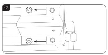
8.4 Undo the 14mm lock nut that holds the pipe to the injector.
