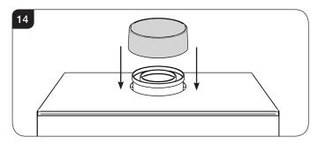
5.13 Connect the flue system, see Installation, Section 6.
