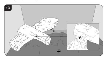
7.5 Place log C on the centre of the burner tray. There is a raised stud in the fuel bed which securely locates the left hand side of the log in place whilst the right hand side rests in the channel to the right hand side of the air cutout in the fuel bed, see Diagram 14.
