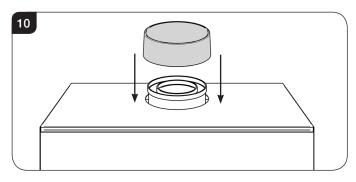
4.12 Connect the flue system, see Installation, Section 6.
