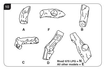
7.2 Place log A on the left hand front of the burner. The log will rest in a groove and the raised stud will fit in the cut out notch in the log, see Diagram 11.
