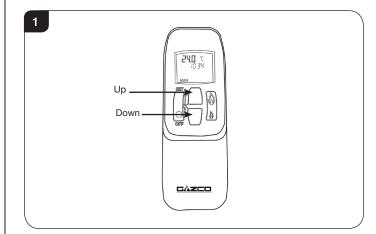
2.1 **Turning the appliance On** Your remote can control the gas appliance from pil
