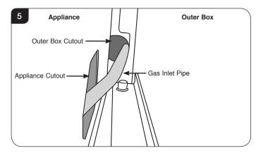
2.8 Feed the pipe through until it exits through the cutout on the right-hand rear of the outer box, see Diagram 6.
