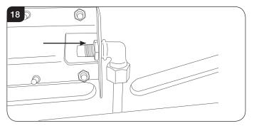
8.5 Replace the injector. Check all joints for gas leaks.
