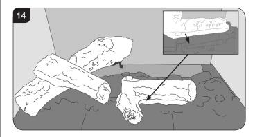
7.6 Rest log D on the raised stud on log C. The rear of the effect should rest against the back liner, see Diagram 15.
