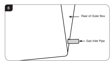
2.9 Connect the Inlet Pipe Extension compression elbow to the appliance Inlet Pipe at the bottom of the control assembly.
