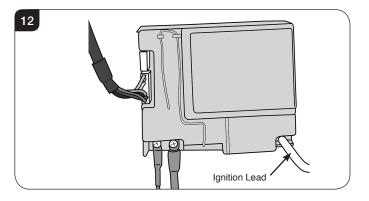
3.14 Carefully cut cable ties and cable ties from the vidaflex.
