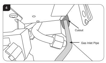
2.7 Carefully feed the pipe between the appliance and the outer box, see Diagram 5.This can be viewed from the front of the appliance, through
