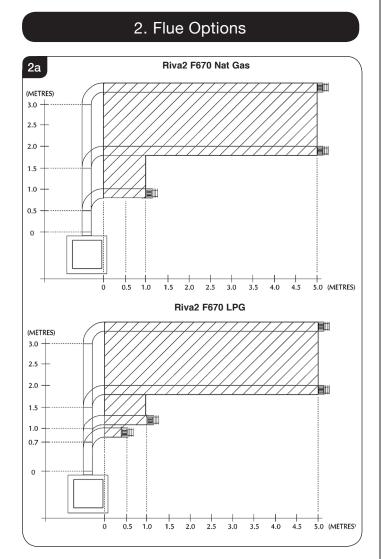
Start of bend to centre line of horizontal flue 170mm. Centre line of vertical flue to end of bend 220mm.
