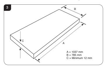
Dimension B allows for a rear clearance of 50mm and a required front projection of 350mm.
