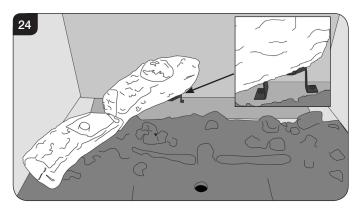
9.4 Place log B on top of log A. There is a hole on the underside of log B which fits over the raised stud in log A to secure in place, see Diagram 25.
