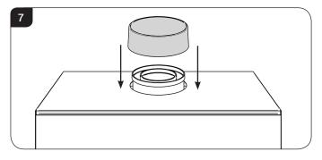
3.5 Connect the flue system, see Installation, Section 6.
