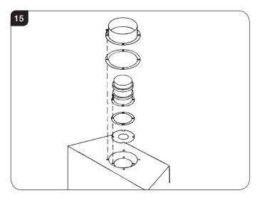
6.2 A 152mm (6") diameter hole is required to install the flue.
