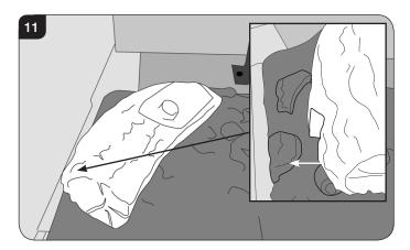
7.3 Place log F behind the first log and locate the rear of the log on the metal bracket. The log should rest between the lip of the bracket and the rear liner, see Diagram 12.
