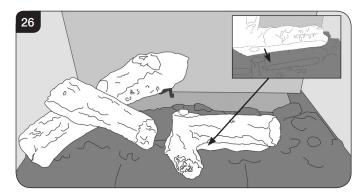
9.6 Rest log D on the raised stud on log C. The rear of the effect should rest against the back liner, see Diagram 27.
