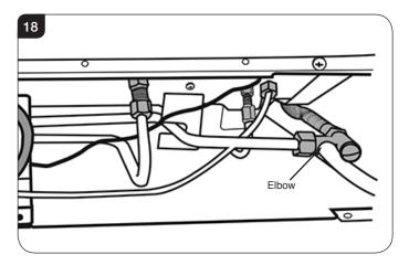
7.2 Connect a suitable pressure gauge to the test point located on the inlet fitting and turn the gas supply on. Light the appliance and check all gas joints for possible leaks. Turn the appliance to maximum and check that the supply pressure is as stated on the databadge. Turn the gas off and replace the test point screw, turn the gas on and check the test point for leaks.
