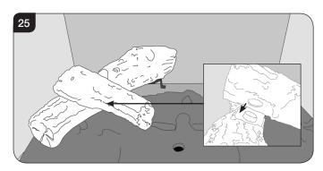
9.5 Place log C on the centre of the burner tray. There is a raised stud in the fuel bed which securely locates the left hand side of the log in place whilst the right hand side rests in the channel to the right hand side of the air cutout in the fuel bed, see Diagram 26.
