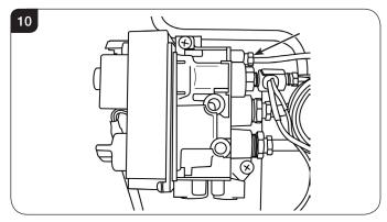
3.9 Remove the pipe and the injector drops out from the burner.
