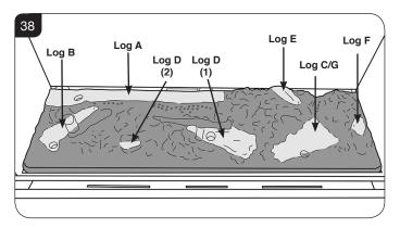
11.4 Place log C (Nat Gas) or G (LPG) on the right hand side of the burner, see Diagram 20. The log will rest on the flat location point shown in Diagram 39.
