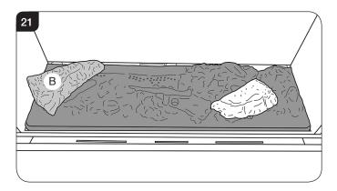
6.6 Place log A behind log B. The log will rest on the flat location plain shown in Diagram 19 with the left side against the left liner and the back against the rear liner, see Diagram 22.
