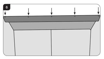
3.3 The Baffle can now be removed by lowering the front edge and pulling forward through the front of the appliance.
