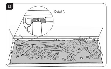
4.6 Slide the Burner Tray to the right, pull slightly forward and lift from the back. Carefully remove through the front of the appliance. Place carefully to one side.
