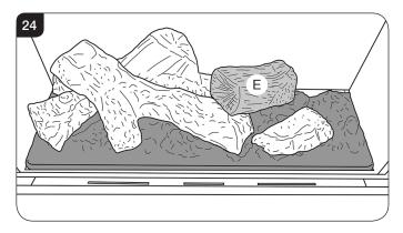
6.9 Position the right hand end of log F on the location point on the burner, see Diagram 19. Rest the left hand end of the log across the back end of log E, see Diagram 25. The back edge of log F should rest against the back liner.
