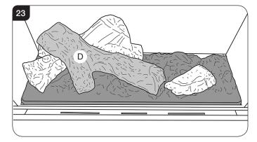
6.8 Position the charred end of log E on the location point on the burner, as shown in Diagram 19, with the log touching the back liner. The front end of the log should rest across the right hand end of log D, see Diagram 24.
