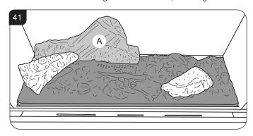
11.7 Position the right hand end of log D on the flat location plain on the burner, as shown in Diagram 38, Log D (1). Rest the left hand end of the log across log B, see Diagram 42. Ensure that the front branch rests in the location point on the burner, as shown in Diagram 38, Log D (2).
