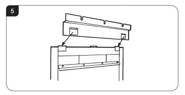
3.2 Secure the bracket to the outer edge firebox using the two clips provided, see Diagram 6.
