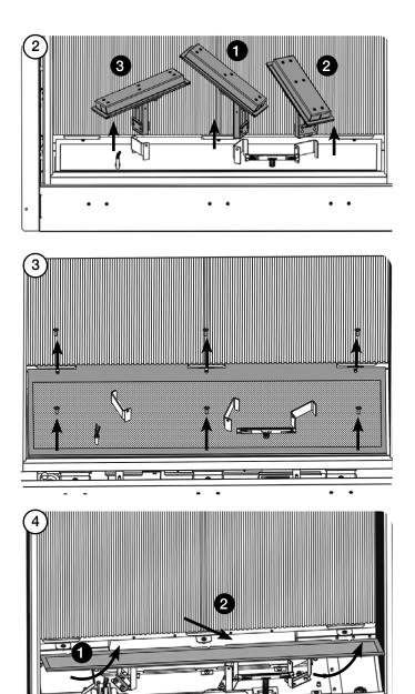
WHEN REPLACING THE MESH TRAY TAKE CARE NOT TO DAMAGE THE LOG BURNER BRACKETS, PILOT AND CROSS LIGHTER. REPLACE THE FRONT SCREWS FIRST BEFORE TIGHTENING THE REAR SCREWS.
