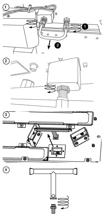
Replace with the correct size Injector and refit all components in the reverse order.
