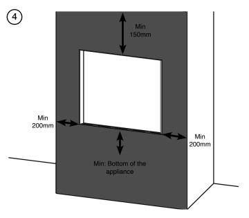
Fit plasterboard to the remaining of the chimney breast front.
