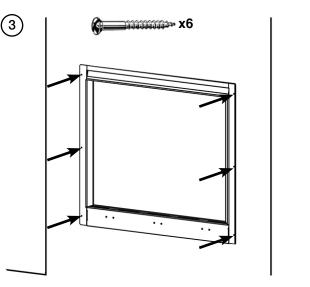
Fit non-combustible board to the chimney breast around the appliance, using the distance to combustibles detailed
