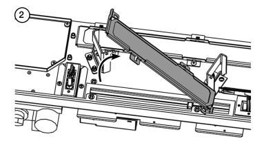
Remove the 2 screws holding the LED boards to the Control Assembly by inserting a screwdriver through the gap previously covered by the glass bracket.
