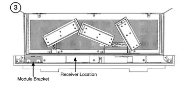
The receiver is located beneath the Main Control Assembly, close to the pilot area.
