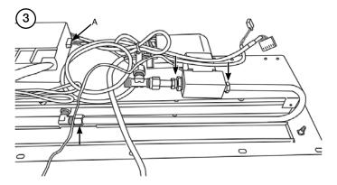
Remove the Solenoid plug from the Control Box (A).
