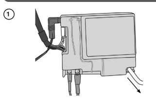
Carefully cut cable ties from the vidaflex and disconnect the lead from the electrode.
