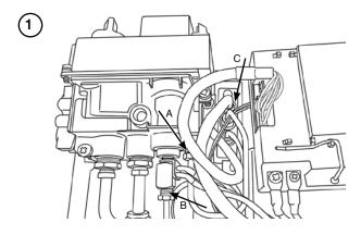
The pilot bracket can now be withdrawn from its cradle.
