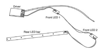
THE LED'S ARE FRAGILE. HANDLE WITH CARE. ONLY HOLD THE LED BOARDS BY THE EDGES TO AVOID CONTACT WITH THE TOP OF THE LED'S. AVOID CATCHING ANY DELICATE WIRES WHEN
