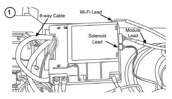
Remove the Ignition Lead. The Control Box is held on by Velcro pads.
