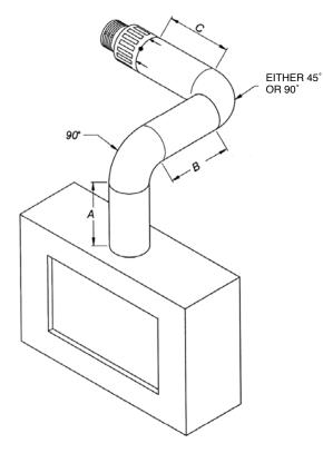
When A = 1.0 to 1.499 metres B + C = 1.0 metres maximum When A = 1.499 metres to 3.0 metres B + C = 4.0 metres maximum
