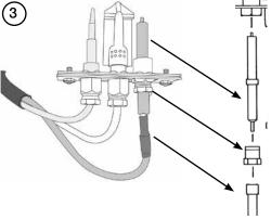
Replace with a new electrode. Do not over-tighten the nut; this could break the component.
