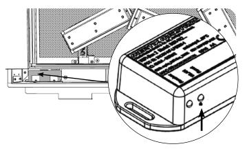
NOTE: Alternatively, the main control assembly can be removed to access the control box, see Servicing Instructions
