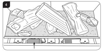
NOTE: Ensure none of the wires are snagged or caught on any internal components.
