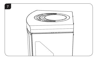
2.11 Secure the cast top plate with the 3 screws previously removed, see Diagram 8.
