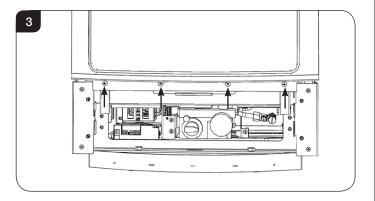
3.4 Lift the glass door slightly and angle the bottom away from the appliance. Lower the glass door to disengage the top hooks from the appliance, see Diagram 4.
