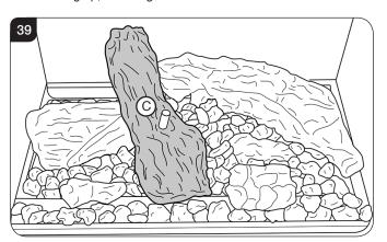
8.7 Log D fits onto the locating pin and rests on Log B, see Diagram 40.
