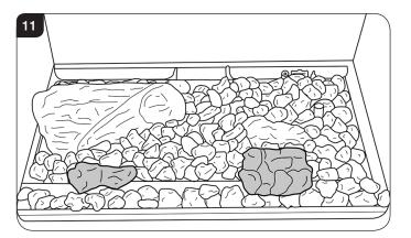
5.5 Log B is positioned on the right hand locating pin, and rests against the back liner, see Diagram 12.
