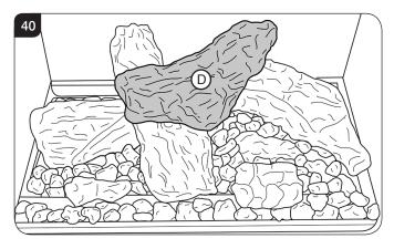
8.8 Sparingly spread an amount of the Embaglow fibres provided on the sections highlighted, see Diagram 41. Take care not to use more than half a packet per application.
