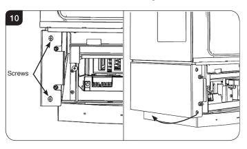
3.4 Pull the front of the side panels away from the appliance and slide backwards to disengage the back tabs, see Diagram 10.
