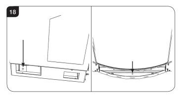
3b.11 Position the appliance on the plinth and secure down through the holes with the screws provided.
