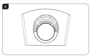
2.10 Replace the cast top plate. When fitted properly the cast top plate should sit flush with the rear of the appliance, see Diagram 7.
