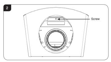
2.6 Remove the flue collar adapter supports and the flue spigot by removing the 4 screws, see Diagram 3.
