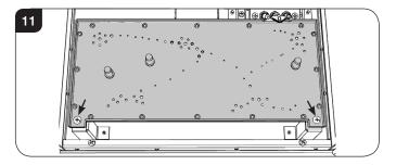
4.2 Lift the burner out of the firebox at an angle clear the brackets, exposing the service hatch, see Diagram 12.
