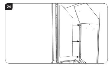
12.3 Replace the glass and gasket, ensuring that the printed side is facing outwards.
