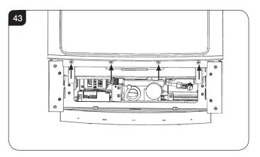
9.4 Replace ALL of the securing screws, ensuring that a screw is present in all fixing slots.
