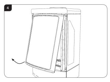
The glass door must be refitted to the appliance following cleaning or servicing.
