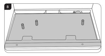
5.2 Place Log A in position on the 2 locating pins, see Diagram 9.
