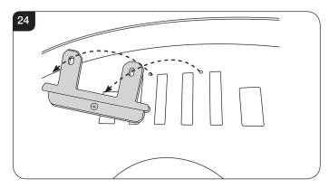
4.6 Fix bracket in the groove on the top of the appliance and secure with a screw, see Diagram 25.
