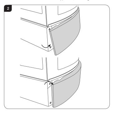
The glass door will need to be removed to gain access to the fuel effect.
