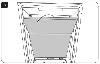
To make removal of the rear panel easier, it may be necessary to remove the burner tray, see Section 4.
