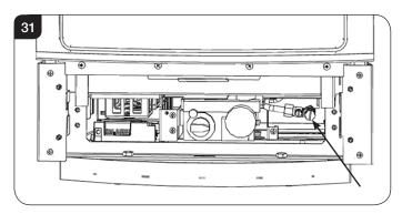
6.2 Connect a suitable pressure gauge to the test point located on the inlet fitting and turn the gas supply on. Light the appliance and check all gas joints for possible leaks. Turn the appliance to maximum and check that the supply pressure is as stated on the databadge. Turn the gas off and replace the test point screw, turn the gas on and check the test point for leaks.
