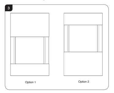
The Support Frames have locating tabs on both the top and bottom to enable them to be positioned either above or below the appliance in order to achieve the desired effect.
