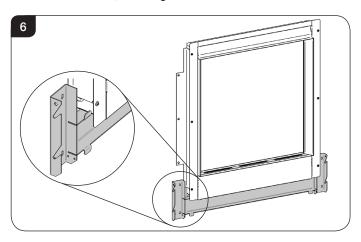
Ensure the Support Frame is the correct way up, see Diagram 6.
