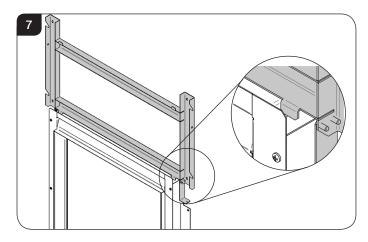
Ensure the Support Frame is the correct way up, see Diagram 7.
