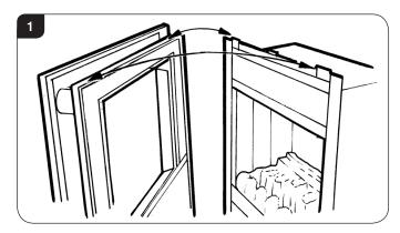
2.2 Place the back of the frame over the locating areas and push down to ensure rigid fixing.
