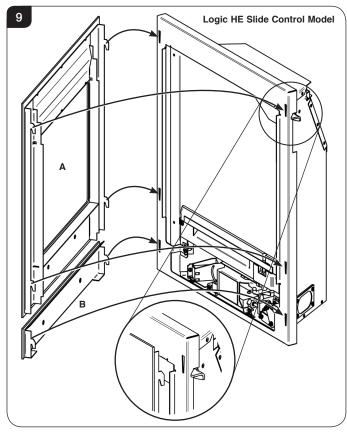
To fit the bottom section/ control cover:
