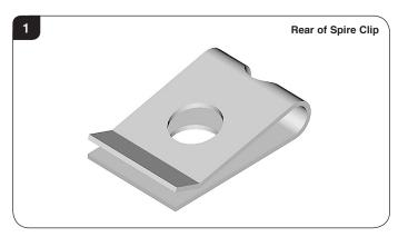
These allow the screws provided to hold the sub frame securely in position.
