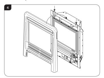
3.4 Secure frame at base with fixing screws as shown to ensure rigid fixing, see Diagram 5.
