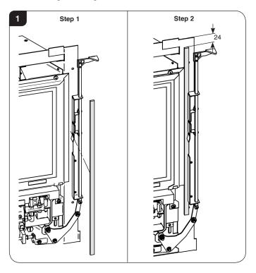
The foam seal must align with the right hand side of the glass frame and 24mm below the top of the appliance flange.
