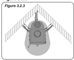
**Scenario I)** Stove in enclosure system using top flue outlet and either single skin or insulated flue. Enclosure is in a corner position at 45 degree angles to each wall: see *Figure 3.2.4*
