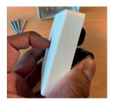
2 Push and hold the front button of the room temperature sensor, while inserting the last battery - do not release the button. When a beep sounds from the room temperature sensor, you may release the button.
