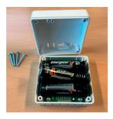
Remove the cover from the room temperature sensor and insert 2 of the 3 AA batteries.
