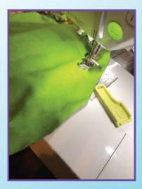
Step 5: Use the Clip 'n Glide Bodkin to insert ribbon into the casing. Once ribbon is inserted, place a bead to hold both sides of the ribbon together. Knot the ends of the ribbon together. You can now gather your pouch or open and lay flat!!!!
