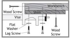
Figure 2 - Mounting Vise to Workbench with Shim
