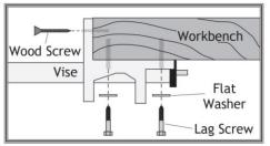
Figure 1 – Mounting Vise to Work Bench
