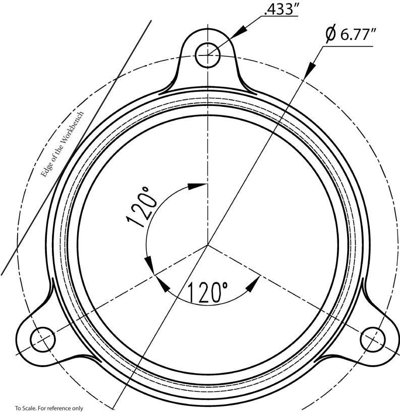
Do not drill holes into the work table until you have received your vise and marked the holes using the mounting tabs on the vise.
