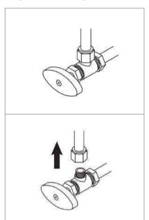
**Locate Shut off valve.** Turn off the COLD water shut off valve located under the sink.
