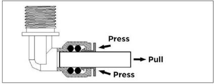
How to release a tube from a quick-connect.
