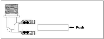
How to insert the tube into a quick-connect.
