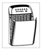
Place the new filter into the air purifier making sure it is facing the correct direction. Airflow travels from outside to the center of the unit. Reinstall the rear cover After replacing the filter, plug the power cord back into an electrical outlet, then hold down the filter button for 3 seconds to reset the filter timer, the indicator light will flash 3times then go out, showing the reset was successful. (See Page 8).
