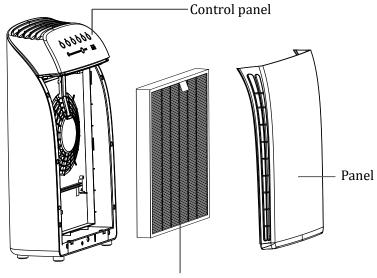
HEPA plus activated carbon composite filter
