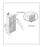
Before using the air purifier for the first time, open the rear cover and remove the composite filter. Make sure to remove any packaging from the filter element, or the product will not function correctly.
