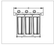
Measure the length (shown as X on diagram) across assembled fittings and subtract 2-inches (50 mm) if you are installing on 1 inch (25 mm) pipe(one inch per side for threads). Mark section of pipe to be removed.
