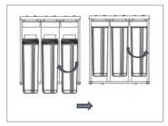
Use the wrench to unscrew the filter bowl, take out the filter cartridge, remove the protective film and label, insert the filter cartridge into the filter bowl, and then screw it tightly.
