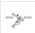
Using a pipe cutter or hacksaw, remove the marked section of the pipe. Remove burrs to ensure a smooth surface without scratches. Align filter assembly with ends of the pipe, making certain filter head port marked "IN" is facing the incoming water supply. Connect to existing pipework.
