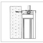
After the housing has been plumbed in, carefully hang the machine on the pre-installed screws.It's essential the housing is secured by the bracket and not just the pipework to support the housing's operating weight when full of water and to hold the filter head tightly when using the filter bowl wrench when replacing filters.
