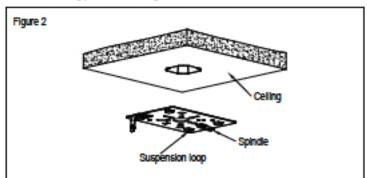
4.lock the M4 screws to complete the Intaliation.
