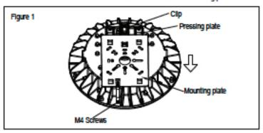
3.Connect the cip on the fixture to the spindle of the mounting plate to make sure the fixture will not slip and fail.connect the line voltage to the wires coming out from the fixture following the wiring diagram. Push the pressing plate into the suspension loop on the mounting plate.
