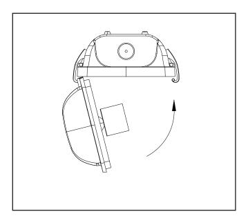
8. Secure lens to housing with lens latches.
