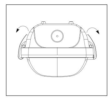
5. Without touching LED boards, detach LED tray and lens from fixture.
