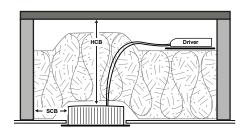
0.5 m Do not install closer than 500mm to illuminated surface
