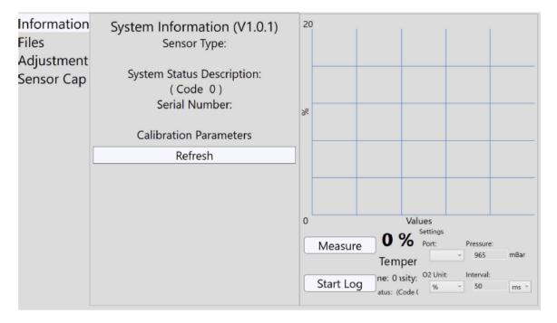
This information is important because it allows you to review the current sensor error codes including the lifetime left for the sensor cap.
