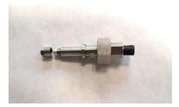
Replace the sensor cap and tighten with a precision torque wrench to 10 Nm (7.38 ft-lbs) of torque. Do not overtighten.
