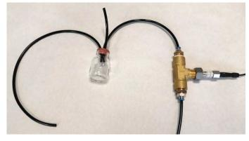
Before you begin calibration, flow the test gas across the sensor for at least 10 minutes to insure that it is fully immersed in test gas. The test gas must always be adapted to the measuring temperature and the sensor flushed with nitrogen without pressure.
