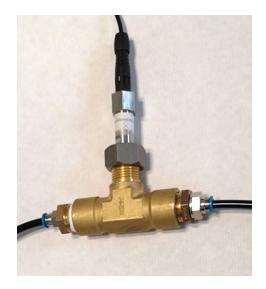
The other end is should be connected to a mechanical pressure regulator set to 100Mbar.
