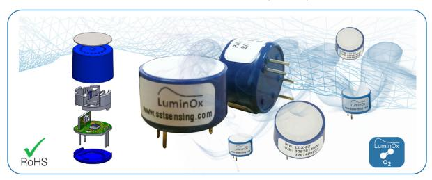
The LuminOx family (LOX) is a range of factory calibrated oxygen sensors which measure ambient oxygen partial pressure ( $ppO_2$ ) levels using the principle of fluorescence quenching by oxygen.
