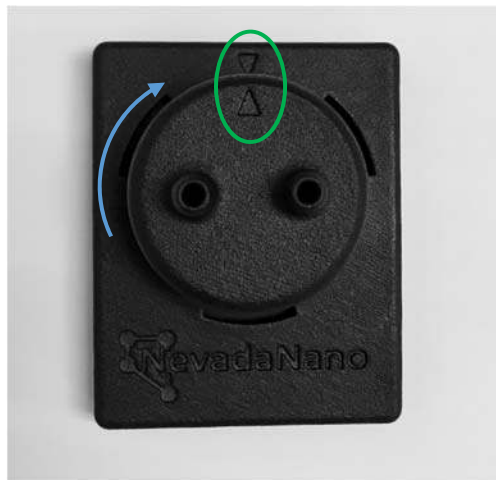
Figure 3 – Proper gas mask attachment is achieved when the arrow points align and the barbs are in the horizontal position.
