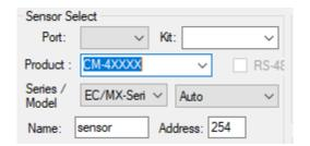
When Gaslab gets the "CM-4xxxx" designation, it questions the EC/MX Sensor, "Are you an Oxygen Sensor"? If the Smart Sensor responds, then Gaslab knows it is an Oxygen Sensor and puts "Oxygen" on the graph. If the sensor does not respond to the Oxygen question, then Gaslab assumes it is a CO2 Sensor and puts CO2 on the graph.
