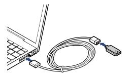
• Insert the sensor into an available port on the USB hub that is connected to your computer.
