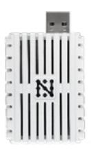
The UA58-KFG-U device has an electrochemical gas(Carbon monoxide, Oxygen, Hydrogen sulfide) sensor and NDIR gas(Carbon dioxide) inside. It transmits measured density information of the four gases(CO, O2, H2S, CO2) in real-time via the USB connector.
