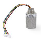
The RG10-NH3-100 is designed to used with RN400-T2GS model for measuring ammonia gas. It is factory calibrated gas sensor that user calibration is not required at all. a whole body would be replaced when the sensitivity goes bad. Individual Certificate is included in the product box. Using UA-Calibration software, RN400-T2GS and gas mixture, a professional customer could calibrate RG10 at zero/span point.
