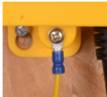
Earth (ground) terminal. Can be used to earth equipment and ducting.
