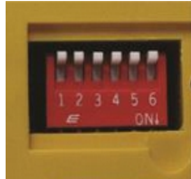
DIP switches – for programming the Pro Switch. All shown positioned OFF factory setting.
