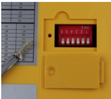
Access panel to DIP switches. Located on the rear of the enclosure. PH1 screwdriver required.
