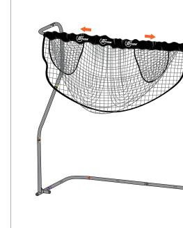
• Once all the tubes are connected, unfasten the Velcro® straps around the net and begin the process of sliding the sleeve down onto the frame, one side at a time.
