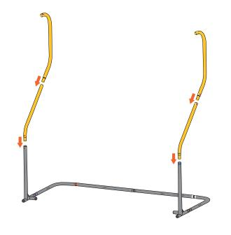
• Continue to build up your frame by connecting the tubes with the identical colored stripes.
