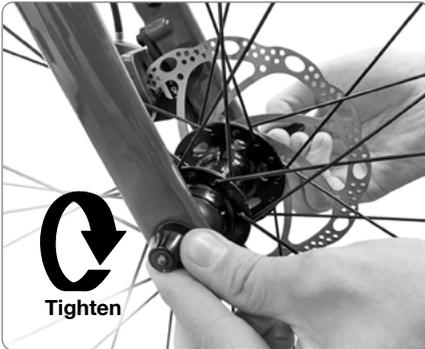
3. Hold QR lever in fully 'open' position and turn nut clockwise. **Do not fully tighten nut.**
