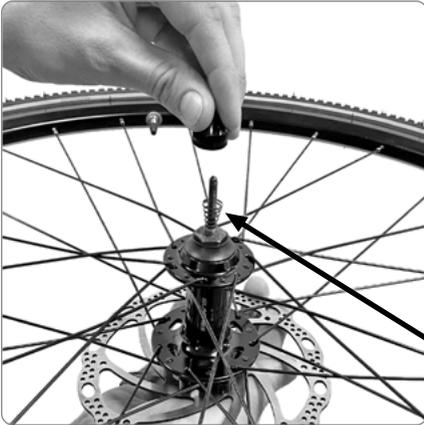
1. Install front quick release (QR) skewer from pedal box.
