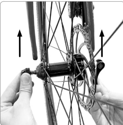
2. Put front wheel into the fork. Ensure (QR) lever is not on gear side. Check this matches the rear wheel.
