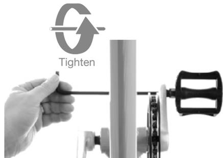
1. Left pedal – rotate pedal axle **clockwise** towards front of bike
