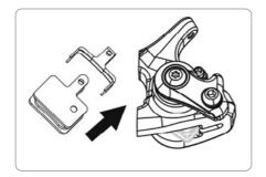
4. Install new pads and spring assembly into the caliper.
