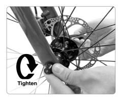
Hold QR lever in fully 'open' position and turn nut clockwise. Do not fully tighten nut.
