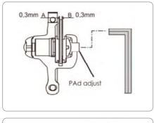
1. Adjust stationary caliper at hub side using 5mm allen key. Turn pad adjustment screw clockwise to move closer to rotor.
