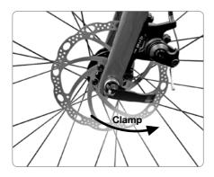
4. Clamp the QR to fully closed position in line with the fork.
