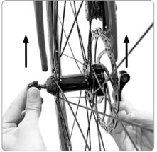
2. Put front wheel into the fork. Ensure (QR) lever is not on gear side. Check this matches the rear wheel.
