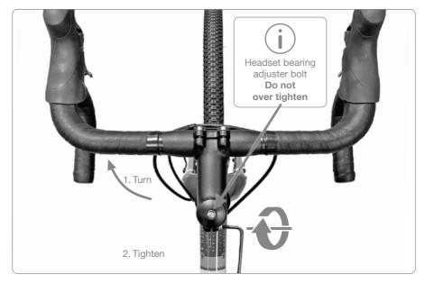
Note: Do not over tighten headset adjuster bolt. This bolt pre-loads i the bearings.
